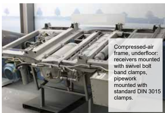
Swivel bolt band clamps to mount the buffer covering
