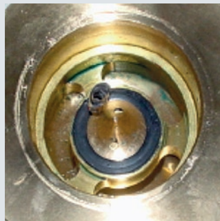
Figure: Damaged valve sealing seat
