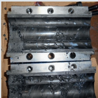
Figure: Damage pump case
