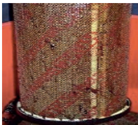
Blocked filter elements
