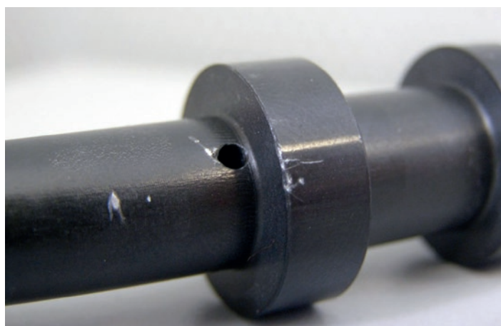
Wear marks on a valve piston
