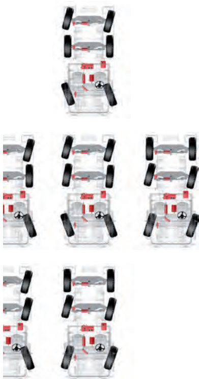
Examples of steering types for two steered rear axles
